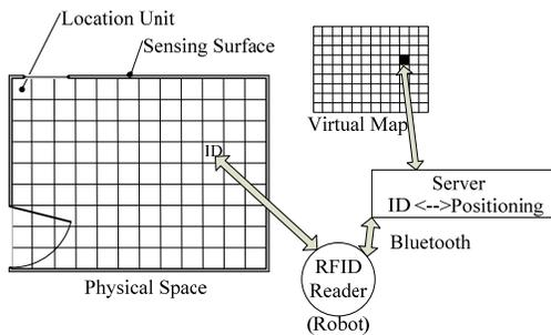
Figure 1. The schematic of the location system concept.
