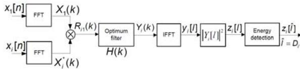
Figure 1. Block diagram of digital TDE receiver.
